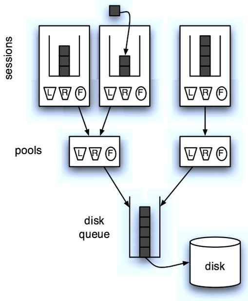
**Figure 2. Token bucket hierarchy and I/O queue structure for sessions, pools, and the underlying device. (R) and (L) are reserve and limit token buckets; (F) is a moving average estimator used for fair sharing.**
