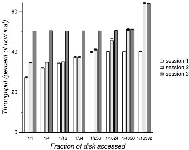
**Figure 3. Fair sharing among streams in one pool. Experiment varied the disk address range that two of the streams accessed to the fraction of the disk shown on the  $x$ -axis, increasing efficiency and making increased performance possible. Results are the average of 10 runs; bars show the 95% confidence interval.**
