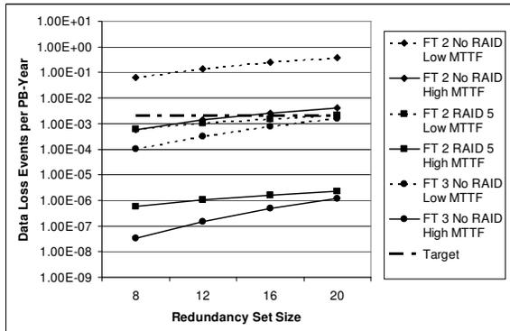
Figure 19: Sensitivity to Redundancy Set Size
