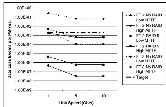
Figure 17: Sensitivity to Link Speed
