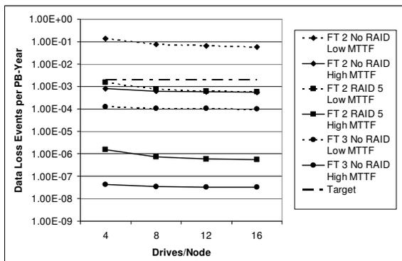
Figure 20: Sensitivity to Drives per Node
