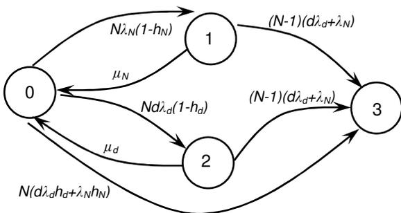
**Figure 8: Markov Model for Fault Tolerance 1; Nodes without Internal RAID**
