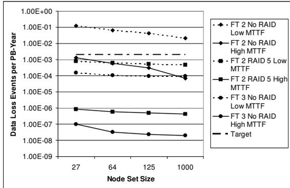
Figure 18: Sensitivity to Node Set Size
