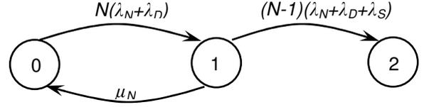
**Figure 5: Markov Model for Fault Tolerance 1; Nodes with Internal RAID**
