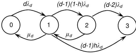
**Figure 4: Markov Model for a RAID 6 array**
