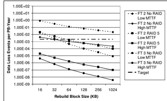
Figure 16: Sensitivity to Rebuild Block Size
