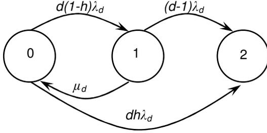
**Figure 1: Markov Model for a RAID 5 array**
