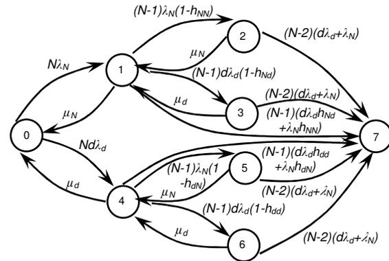
**Figure 9: Markov Model for Fault Tolerance 2; Nodes without Internal RAID**
