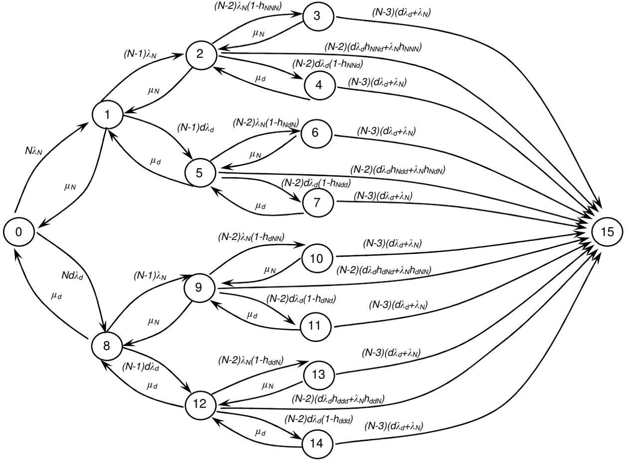
**Figure 10: Markov Model for Fault Tolerance 3; Nodes without Internal RAID**
