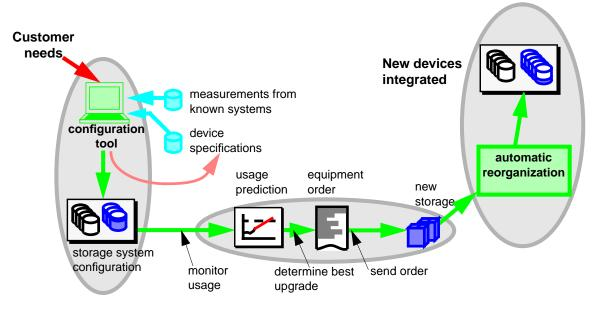
The life-cycle of the self-configuring, self-managing storage system starts with a model of the system workload, based on which the initial configuration is built. The system monitors changes in the workload, not just to order more devices, but also to guide load balancing and rearrangement along the way.
