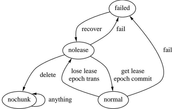
When a chunk is deleted, as part of an epoch transition or by a manager while the chunk is attempting recovery, the chunk goes away. We model the absence of a chunk by the **nochunk** state, which specifies what the device will do when requests are made on a chunk that doesn't exist.
