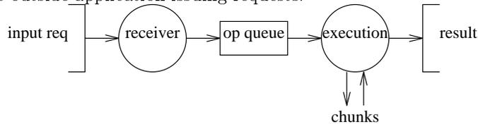
The execution machine in the host uses two BSTs [Amiri99], or patterns of message passing, to perform high-level reads and writes. The patterns are encoded in the execution engine's state transitions.
